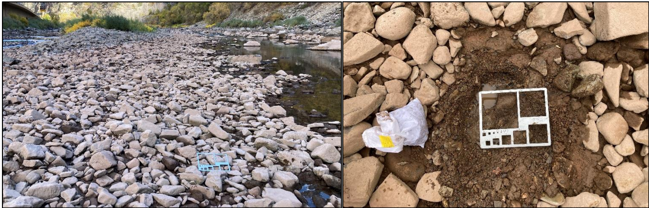
Figure 10. Sediment sample locations at the far downstream end of the channel center cobble bar. Left – area Wolman pebble count was conducted. Right – subsurface sample location with cobble armor layer removed.
