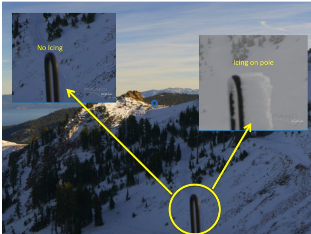
Figure 5. Example of mountain top icing conditions. The yellow circle shows the icing pole. The inset image on left shows the no icing conditions and the inset image on the right shows the results when icing (cloud seeding conditions) are present.
