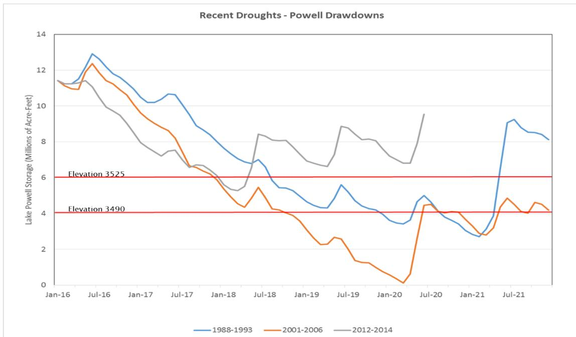
**Figure 1. Past Lake Powell drawdowns superimposed on current conditions. A repeat of any of the last three drought events and subsequent drawdown of Powell would threaten the Upper Basin’s ability to meet its obligations under the 2007 Interim Guidelines. The Upper Basin States and Reclamation have designed a Contingency Plan to keep Powell’s elevation above the 3525’ threshold.**
